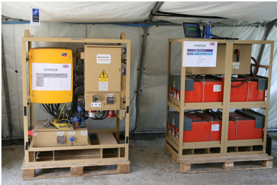
Used by the North Atlantic alliance, this intelligent system which stores surplus energy and distributes it has been known to cut fuel consumption by an average of 30 per cent. Source: North Atlantic Treaty Organization.
